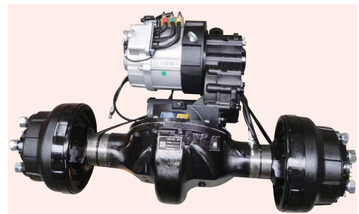
Transverse-Mounted IC-Spec Drive Axle and Transmission.
