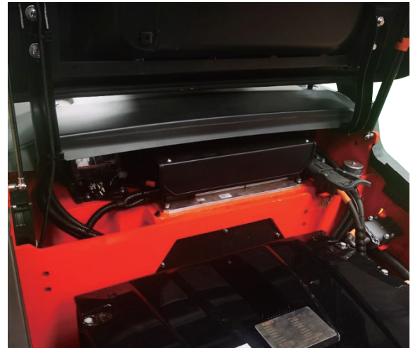
Fully Enclosed Controller Design, Rear-mounted within the counterweight for optimal heat dissipation, water, and dust resistance.
