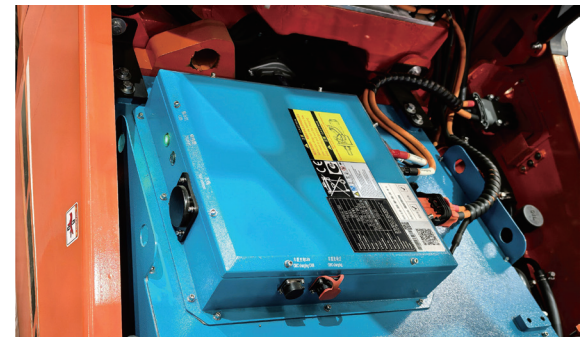
Independently Distributed Cells and BMS.
